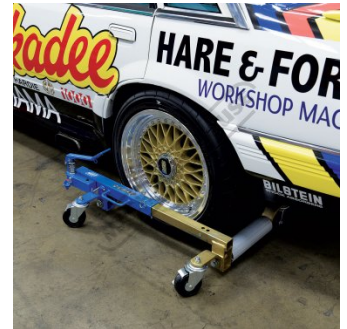
Positioning Jack in Place 2
