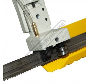
Carbide Blade Guides With Bearings
