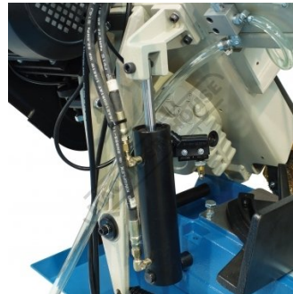
Hydraulic Arm With Automatic Cut Out Switch
