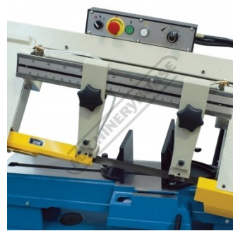
Quick Adjustment Blade Guide System
