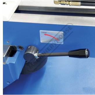
Clamp Vice Position Locking Lever
