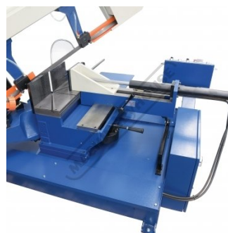
Automatic Full Stroke Hydraulic Clamping Vice
