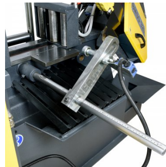
Length Stop Adjustment
