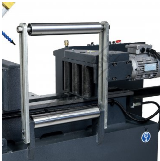
Adjustable Top Roller Support
