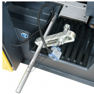
Repetition Auto Length Stop Switch
