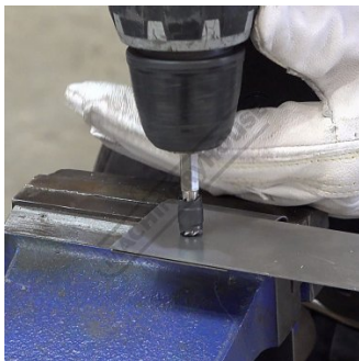
Push Down Ready For Drilling
