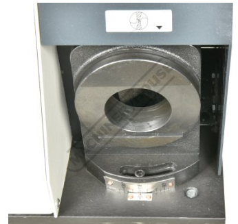
Drill Angle Setting at 90 Degrees
