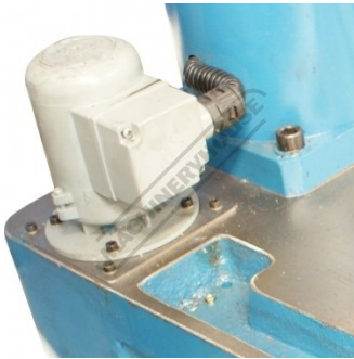
Coolant Pump System
