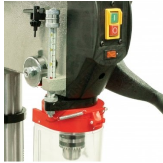
Drilling Depth Stop Setting with Scale
