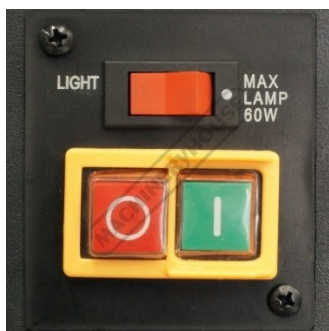
Magnetic Switch and Light Switch
