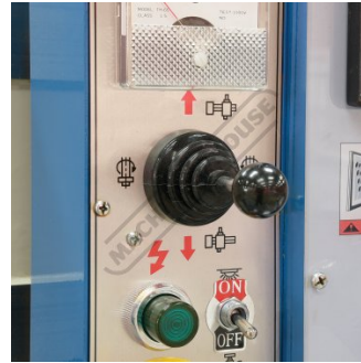
4 Way Joy Stick Control for Arm Rise-Fall-Spindle Direction
