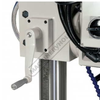
Rack-Pinion Wind Up Drill Head
