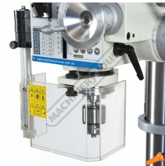
Interlocked Spindle Safety Guard
