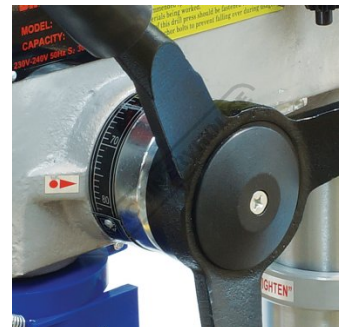
Drilling Depth Stop Setting With Scale
