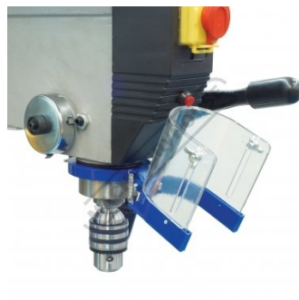
Safety Chuck Guard Flipped Up
