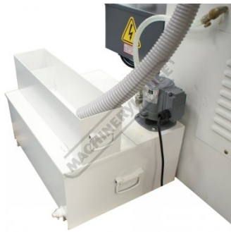
Coolant Tank with Backstop Valve
