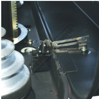
Safety Micro switch on Belt Guard
