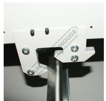
Drawer in Unlock Position
