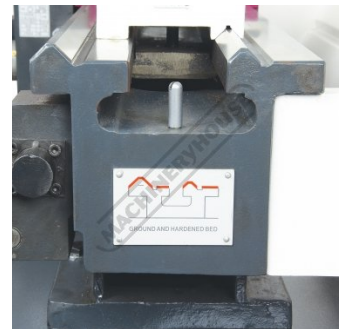
Ground and Hardened Bed
