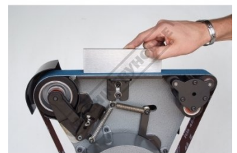
Flat Grinding on Platen
