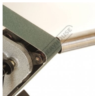
Internal Pipe Chamfering
