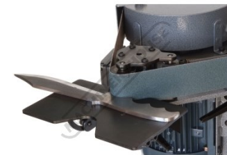
Optional Tilting Table for Contouring & Pipe Notching
