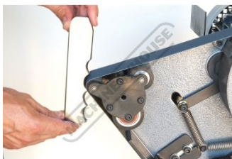
Small Wheel Selection for Notching & Contouring
