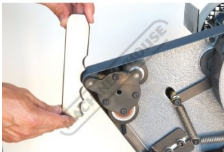
Small Wheel Selection for Notching & Contouring
