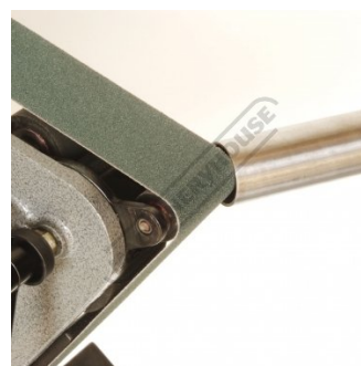
Internal Pipe Chamfering
