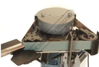
Tilting Table for Contouring & Pipe Notching
