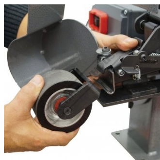
Contact Wheel Removal
