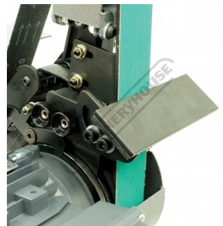
Platen Table Tilted Down
