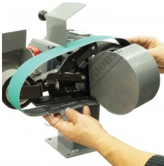
Remove and Replace Belt
