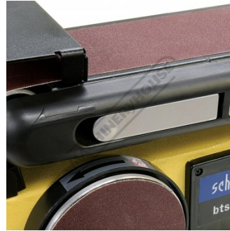
Belt Tension Release Lever
