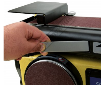
Releasing Tension To Change Belt
