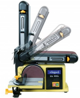
Horizontal to Vertical Finishing
