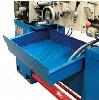
Sliding Drip Tray for Swarf Removal
