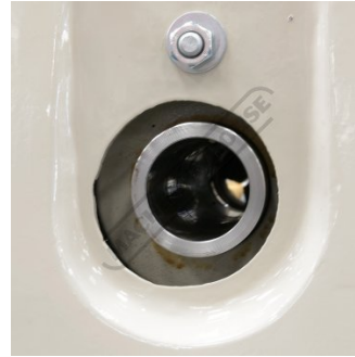
40mm Spindle Bore
