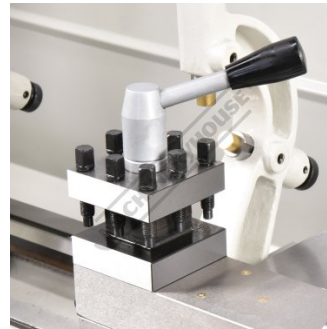
Compound Slide with 4 Way Toolpost
