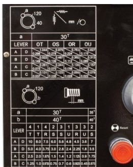
Longitudinal and Cross Feed Chart And Metric Thread Chart
