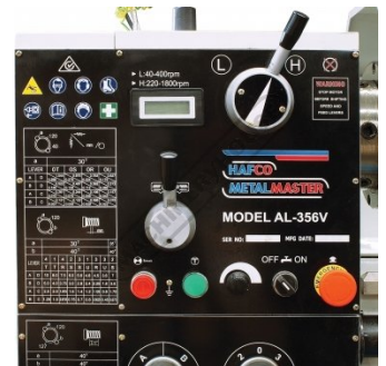
Spindle Speed Controls
