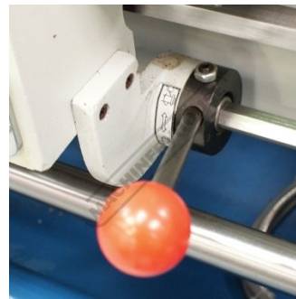
Spindle Engagement Lever
