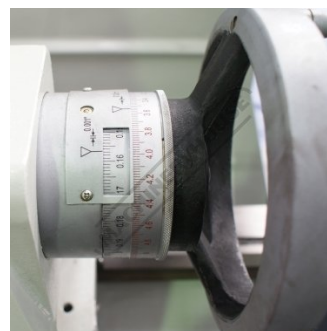
Tailstock Hand Wheel
