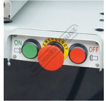
Power Control Panel On Saddle
