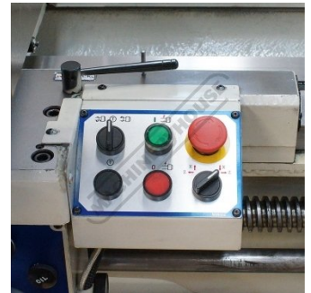
Saddle Switch Board
