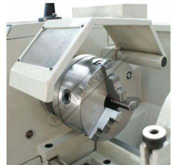
Chuck Guard With Safety Micro Switch
