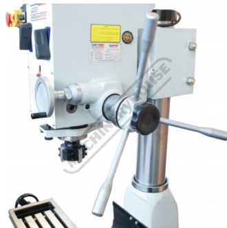
Fine feed handwheel operating quill feed
