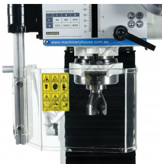
Interlocked Spindle Safety Guard
