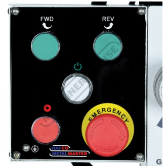
Forward Reverse ON OFF and Emergency Switches
