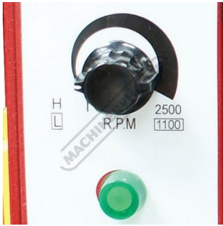
Electronic variable speed system
