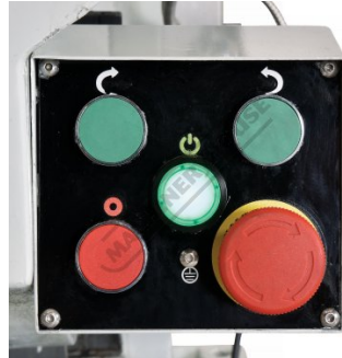
Horizontal Spindle Control Panel
