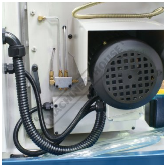
Oil Feeder Distribution Block
