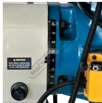
Tilting Mill Head Left & Right to 90 Degrees
