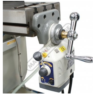
X Axis Power Feed with Rapid
