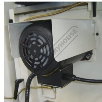
Knee Elevating Motor for Z Axis
