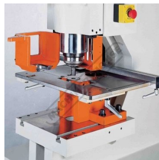
Includes large hole punching up to 50mm Diameter
