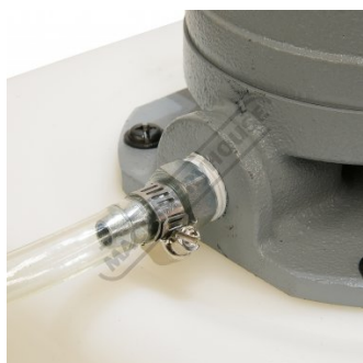
Coolant Pump Flow Outlet
