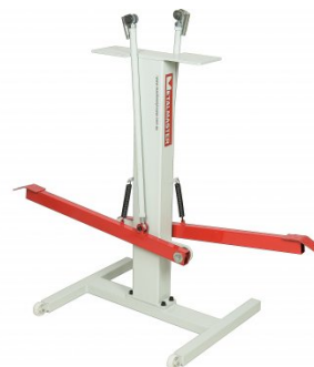
S2263 Shrinker Stretcher Foot Operated Stand
