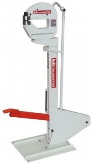
S2266 Foot Operated Shrinker Stretcher - Heavy Duty
