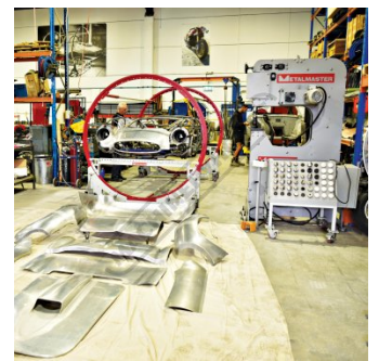
All Car Parts Made on Power Hammer
