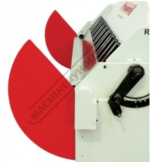
Apron Safety Guards
