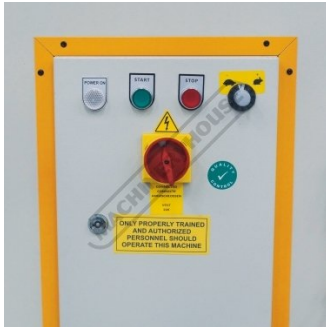
Control Panel with Variable Speed
