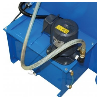
Coolant Pump and Tank
