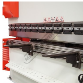
Adjustable and Sliding Front Sheet Supports
