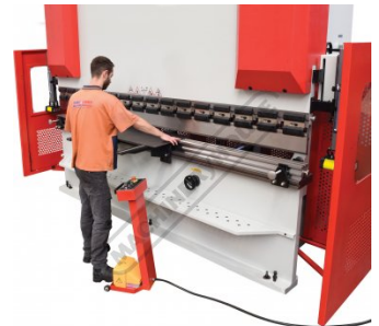
Laser Guarding system In Use
