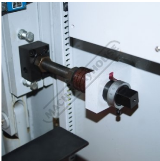
Quick Action Blade Clearance Adjustment
