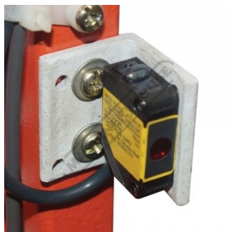
Safety Omron E3ZS Rear Light Sensor Guarding
