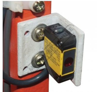
Safety Omron E3ZS Rear Light Sensor Guarding
